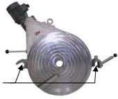
Therefore the eyes must be lubricated with PTFE spray before each transport!
