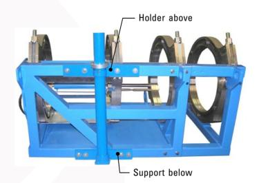
Put the lifting device through the upper holder from above and downwards to the lower support.
