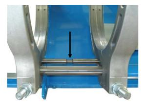
There is a puller mounted between the movable and the fixed clamping shells on the basic machine. It prevents the heating element from sticking to the heated-up pipe ends.
