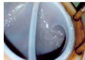
PVDF/Blister is observed (Electrolysis Plant/ Return Brine 88°C, 0.3MPa, after 5years service)
